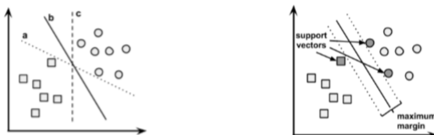
Figure 1 a) hyperplane options of separating the data / b) the Maximum Margin Hyperplane (Lantz, 2013).
